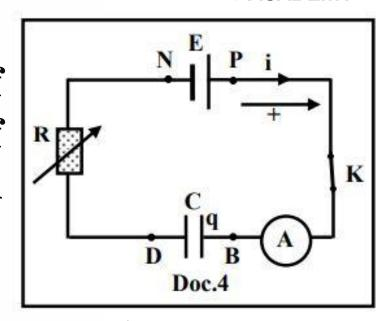
Initially the capacitor is uncharged. We close the switch K at the instant  $t_0 = 0$ .
