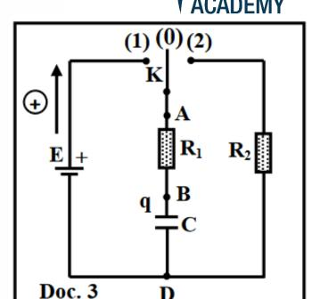
At the instant  $t_0 = 0$ , K is turned to position (1) and the charging process of the capacitor starts.
